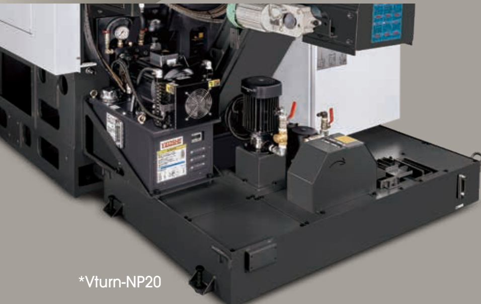
Coolant flush onto covers (Photo with opt. pump Grundfos® MTH 4-4/4)
